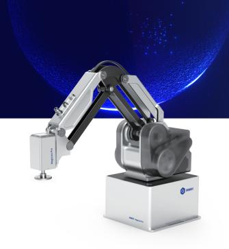
MG400 is a lightweight desktop robot with a footprint smaller than one piece of A4 paper. Designed to be flexible to deploy, easy to use, and safe to collaborate, MMG400 makes automation affordable and accessible for diversified and small-batch production scenarios. Featuring 750g payload, 440mm maximum reach, hand-held teaching and collision detection, MG400 truly fits perfectly for lightweight desktop applications and fast deployment in the production line.
